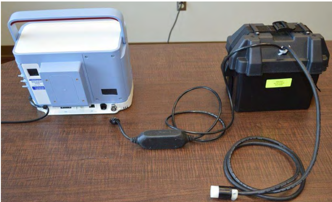
Figure 8. Trilogy Ventilator with 12V marine battery, battery cable- courtesy of the Ventilator Equipment Pool. March 2017
