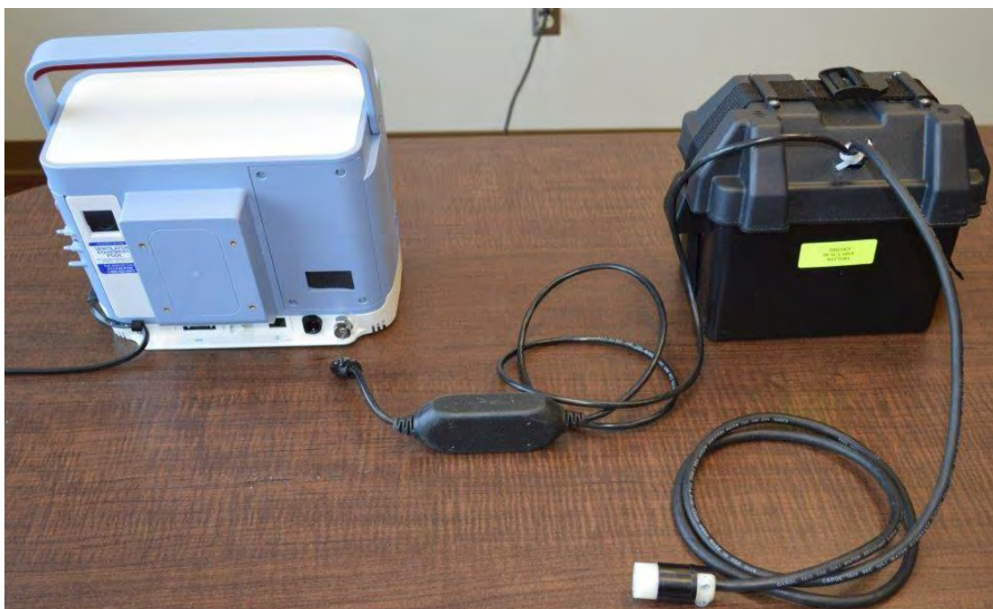
Figure 8. Trilogi Ventilator with 12V marine battery, battery cable- courtesy of the Ventilator Equipment Pool. March 2017
